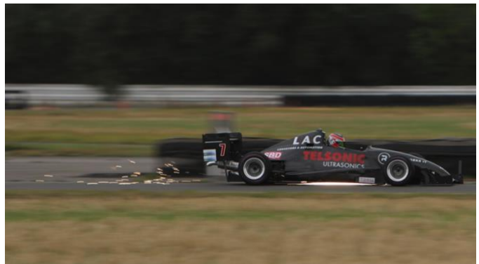
Sparks flying from the titanium skid plates under braking – 2.5G longitudinally. Photo by Kim Broughton
