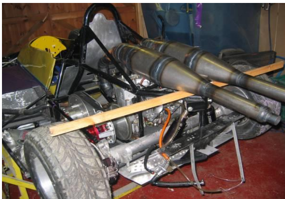
Rotax 600HO engine being fitted with twin expansion chambers in position. Shows solid rear axle within aluminium casing and heavy duty bearings each end
