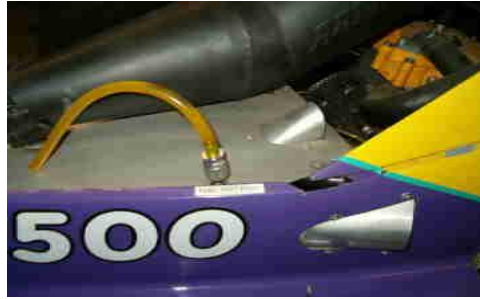
Fuel test port with quick release hose.
