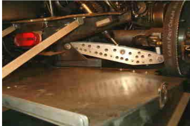
Rebuildable Alum. Swingarm w/hi performance bushings. Rear adjustable Alum defuser panel Semi-Carbon fiber support header, old belt drive.
