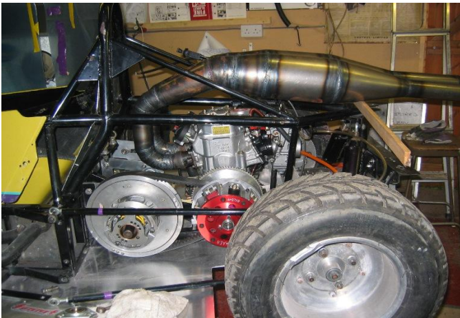
CVT transmission with Aon 4 -Star drive clutch and Polaris driven clutch. Hi-Tech adjustable spring tension Spare weights,springs,belts etc.etc
