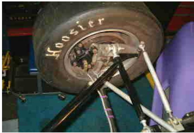
New design frt & rear Wilwood brakes w/quick change pads. 7" vented, slotted rotors. Maverick upper & lower A arms allow for EZ Caster/Camber adjustments. Performance frt end wheel bearings.
