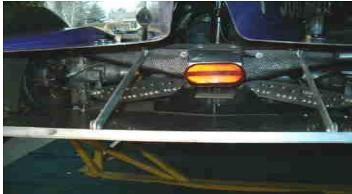
Rain Light. Special alignment clip with alignment poles to square up chassis
