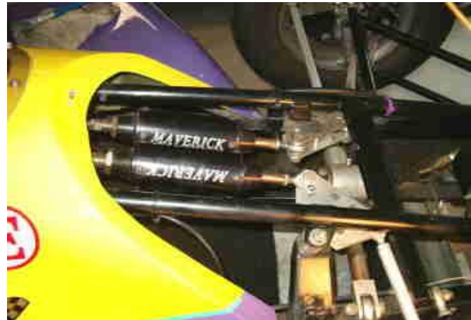
Maverick ft & rear adjustable rebuildable dampeners. " rebuildable performance bellcranks w/Hi performance bushings.
