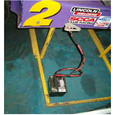
Aux. Battery, cable and hook-up
