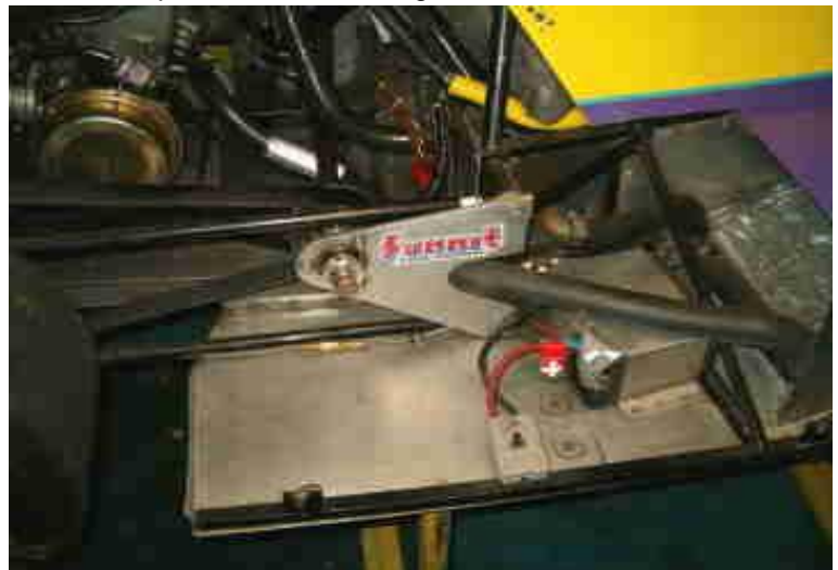
On board new Red Top battery with Auxillary battery hook-up for better starts. Electric starter. Clean plumbing and fuel and water overflow catch bottles. Air Pulse fuel pump.
