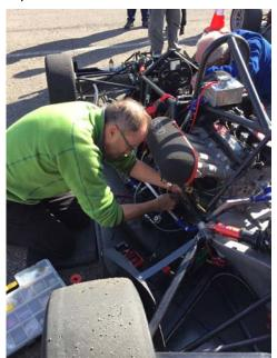
We spent over 2 hours looking for an electrical short between the 0 and 5v lines – perhaps a tiny chaffing. Couldn't find anything. We swapped ECUs from another car, traced every pin to the sensors for continuity, disconnected every sensor. Nothing.
