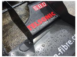
The development to the car continued during the Sunday – progressively increasing the rear ride height with the aim of gaining downforce from the underside of the whole car and reducing the drag by minimising the wing.
