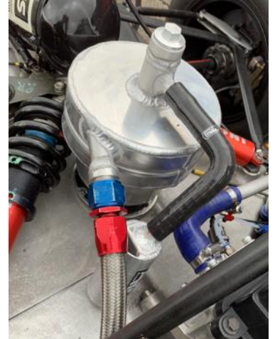
James at ARF work, showing new oil sump tank and catch bottle
